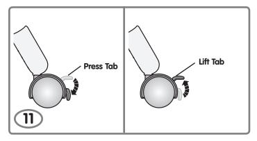
**To Lock:** Press the tab on all four wheels down until you hear a "**snap**".
